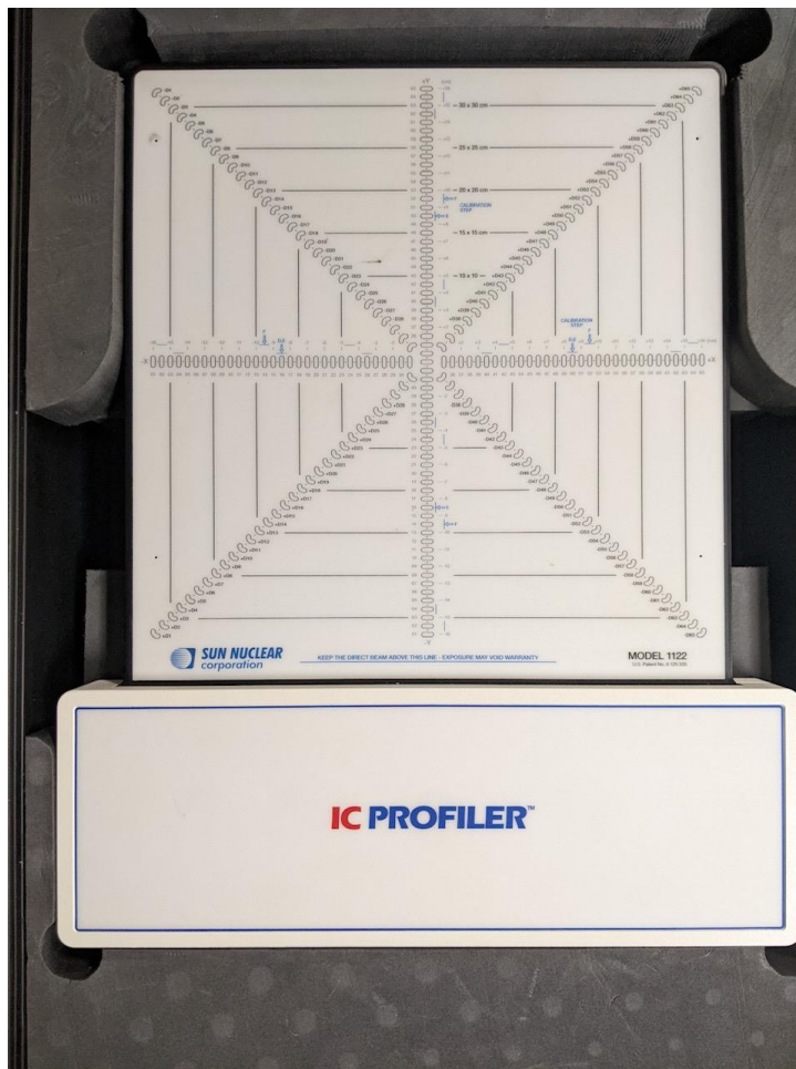
Figure 29. Pictures showing the Sun Nuclear IC profiler used to generate the beam profiles and PDD curves with the central axis.
