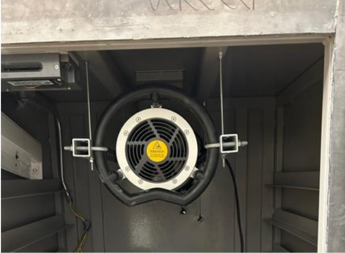
Figure 25. Image of the X-ray tube suspended from the ceiling of the cabinet on all-thread rods that attach to the square aluminum tubes. U-bolts attach the square aluminum tube to the round handles at the front and back of the X-ray tube.
