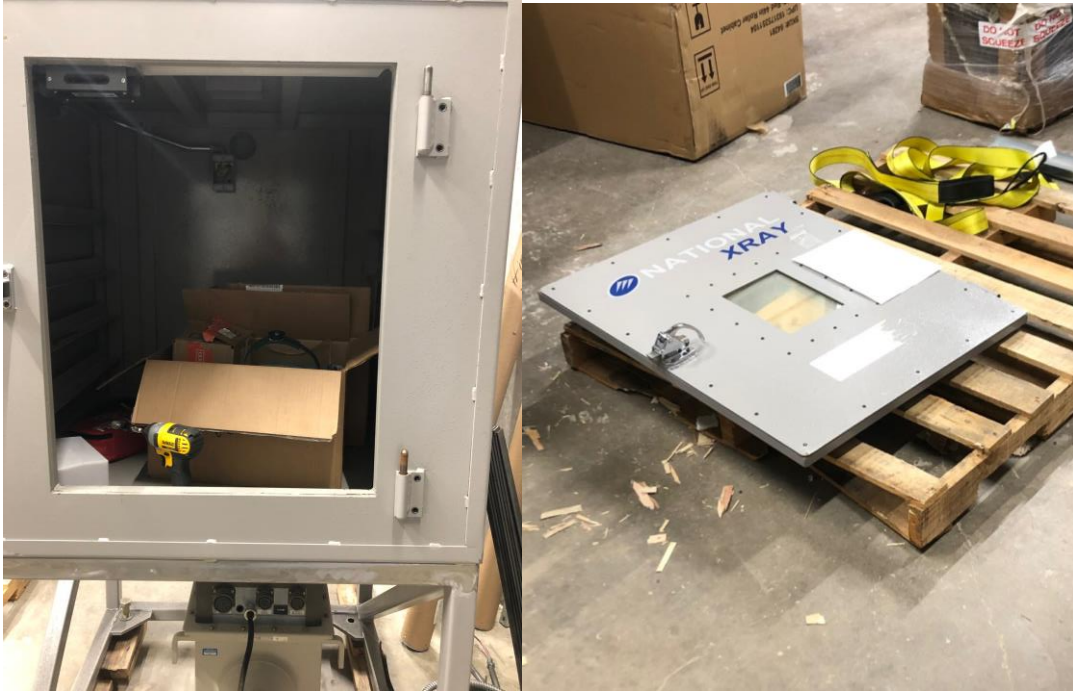
Figure 21. Images of the X-ray cabinet with the door removed and the paint removed from the 2 by 2 in. steel tube at the bottom of the left image. The hinges seen here were also removed.
