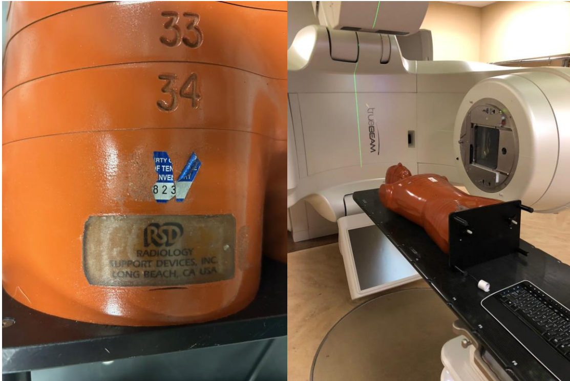
Figure 50. Images of the Radiology Support Devices phantom placed on the couch of a Varian TrueBeam linac. The cone beam CT was used to take radiographs of the phantom for comparison with the 300 keV X-ray tube imaging.
