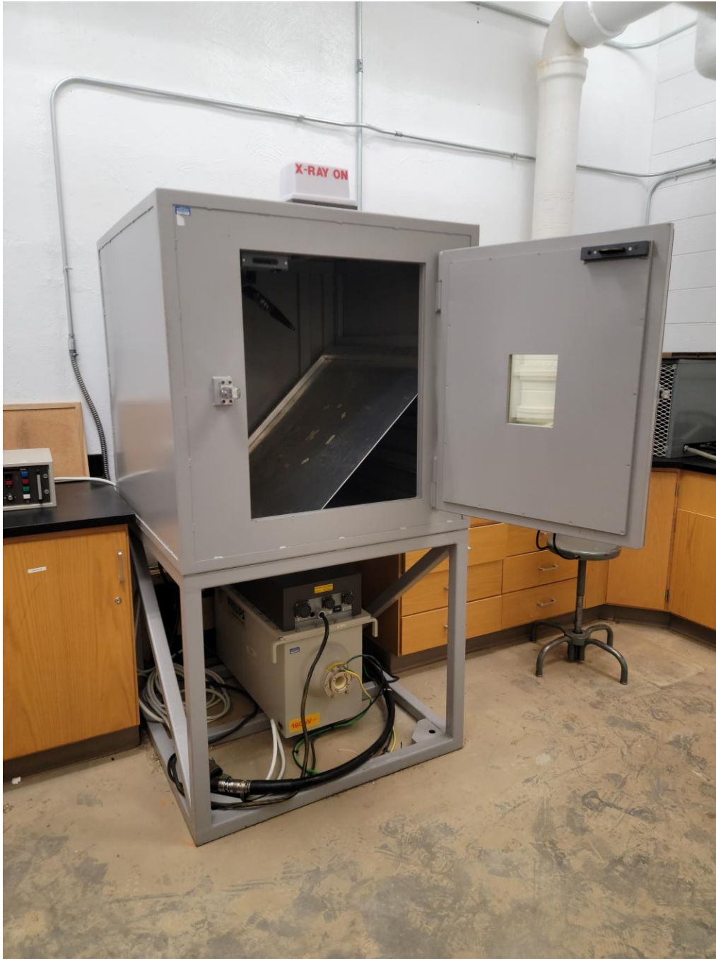
Figure 16. Image of the national X-ray radiation cabinet used as the basis for the NCRP calculations and the MCNP shielding simulations.
