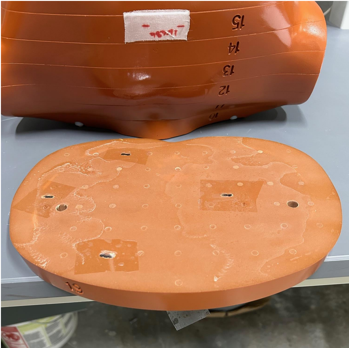
Figure 52. A cross-sectional layer of the RSD phantom with the nanoDots embedded in the plastic at different locations. They are covered in tape so they do not fall out when the layer is placed back on the main body of the phantom in the background of the picture.
