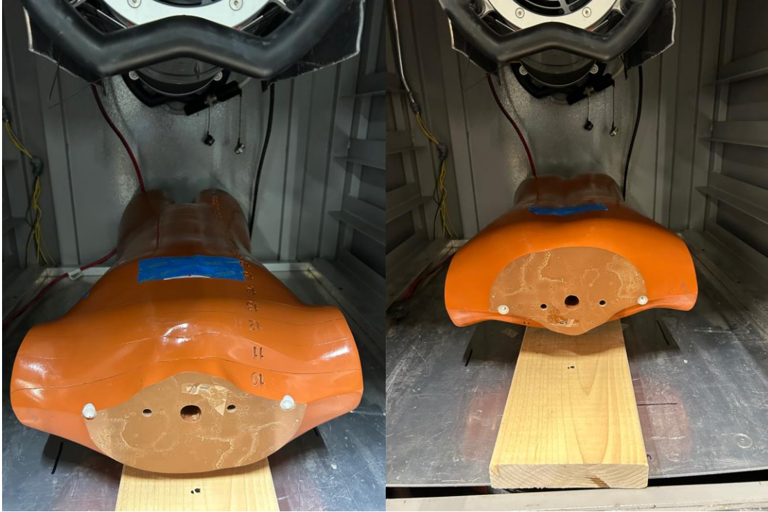
Figure 60. The left image is the AP field setup, and the right image is the PA field setup. The wooden board acts as a spacer to ensure the SSD is 35 cm. The beam's central axis is underneath the blue tape, containing the surface dose nanoDots.
