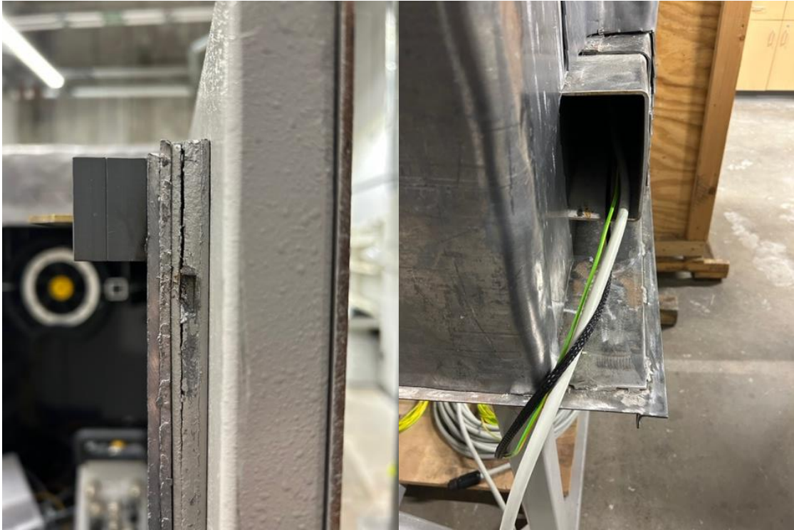
Figure 24. Images showing the addition of lead sheets to the inside face of the door with the interlock blade installed. The right image shows the cable chase and cables routed to the inside of the cabinet.
