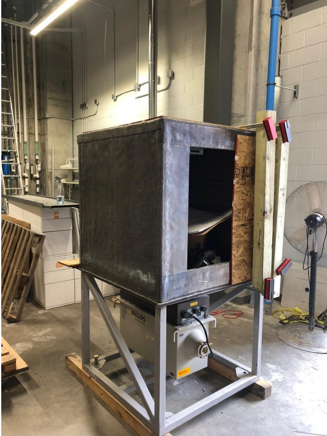
Figure 23. Image of the X-ray cabinet with the lead sheet held in place with wood 4 by 4 in. posts and plywood to apply even pressure. Notice the overlapping seams along the edges.
