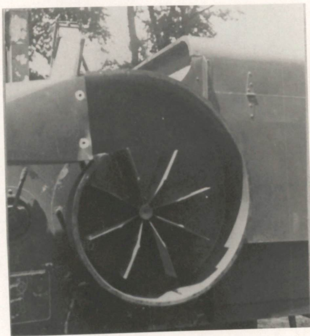
Figure 6. Fan with Cover Removed
