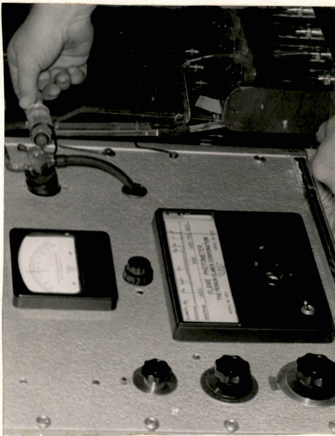
Figure 1. Potassium determinations made direct from soil extract in filter tubes by using four-way stopcock connected to atomizer on flame photometer.
