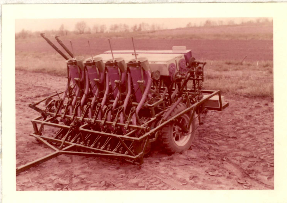
Figure 1. Special experimental drill developed by the United States Department of Agriculture, Agriculture Research Service, Agricultural Engineering Research Division and used for seeding and fertilizing experimental plots.
