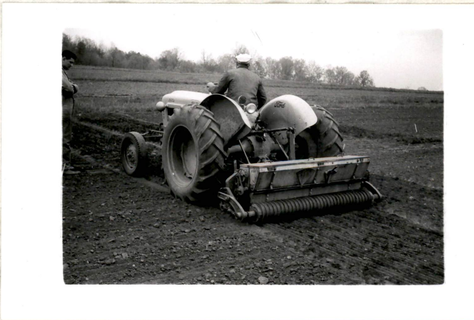
Figure 4. View of "Brillion" double-corrugated roller used in firming plots where seed alone, or both seed and fertilizer were broadcast.
