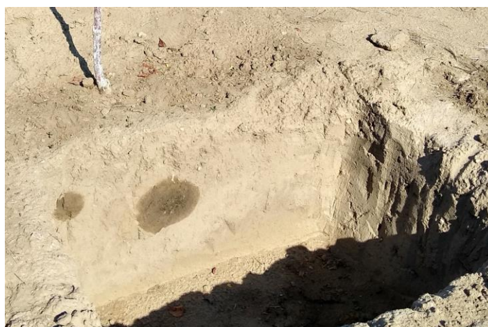
Figure 7. Soil profile with the wetting pattern in variant with horizontal SLECI – Jul-2020.
