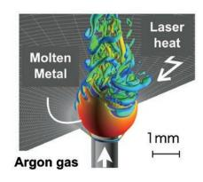
液滴浮遊法の流体構造連成解析 Fluid-structure interaction analysis of a gas-jet levitation method
