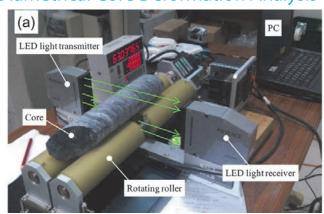
特別に開発したコア変形測定装置 A newly developed apparatus for measuring circumferential distribution of core diameter.
