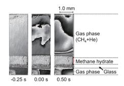
メタンハイドレート分解における固気界面近傍の輸送現象の可視化 Visualization of transfer phenomena near the solid-gas interface during methane hydrate decomposition
