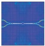
Crack propagation by particle method
