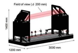
大型干渉計外観 Exterior of large-scale interferometer
