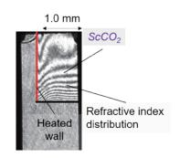
超臨界二酸化炭素中における熱輸送現象の可視化 Visualization of heat transfer phenomenon in carbon dioxide under supercritical condition (ScCO<sub>3</sub>)
