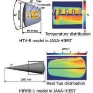
極超音速飛行体の空力加熱計測 Aerodynamic heating of Hypersonic airplane
