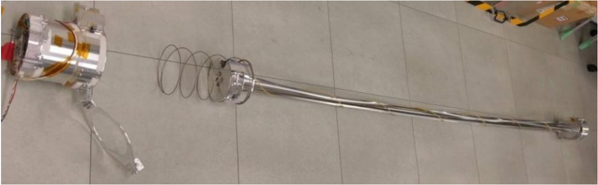
Figure 3.35: Fully extended boom of SDOM after separation from the main cylinder with an undeployed sail. (©JSASS)
