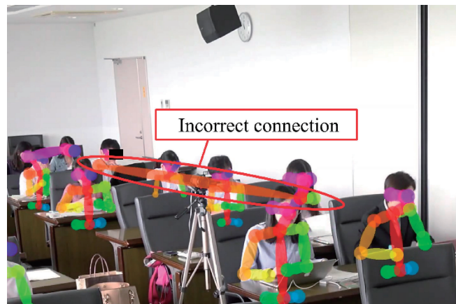
Fig. 7. Example OpenPose output. Detected keypoints from several persons are connected incorrectly, as indicated by the red circle.
