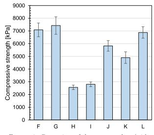
FIGURE 4. Comparison of the average values (with standard deviations) of the compressive strengths of the tested gypsum mixtures.
