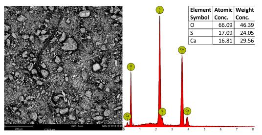
FIGURE 2. Chemical analysis of recyclate by SEM EDS analysis.
