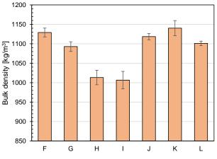
FIGURE 3. Comparison of the average values (with standard deviations) of the bulk density of the tested gypsum mixtures.
