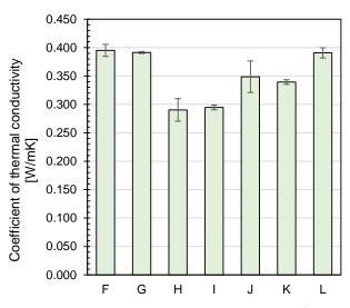
FIGURE 5. Comparison of the average values (with standard deviations) of the thermal conductivity coefficient of the tested gypsum mixtures. The values were determined for naturally moist samples in a laboratory environment at a temperature of  $25\pm2$  °C and a relative humidity of  $50\pm3$  %.
