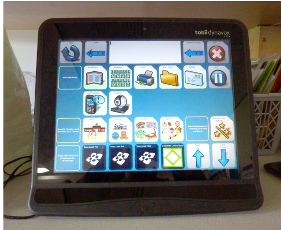
Figure 2.2: Tobii Dynavox SGD featuring Communicator 5 software with eye tracking access, photographed during Study 1 of this project.
