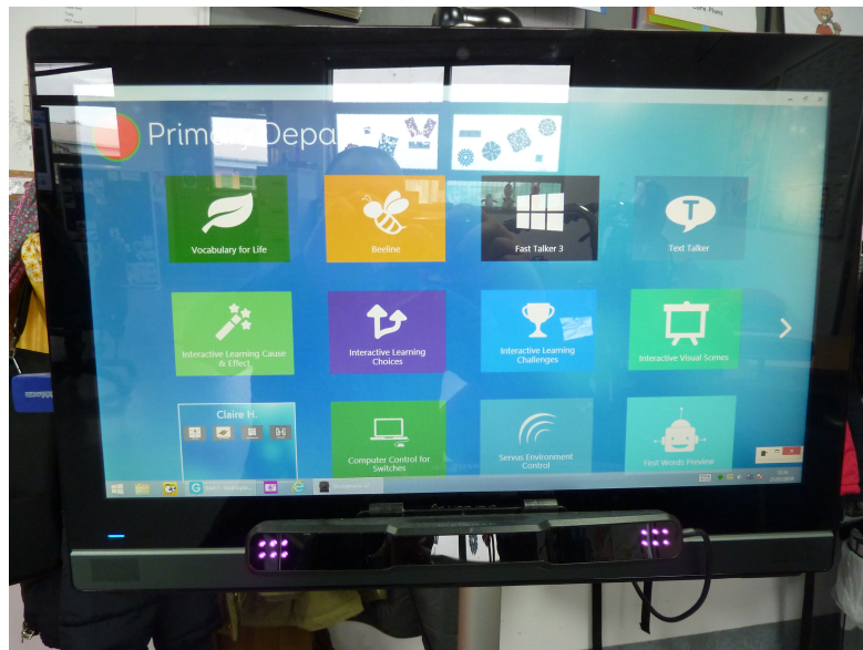
Figure 4.9: Standalone touchscreen PC on a floor stand with eyegaze hardware in class.
