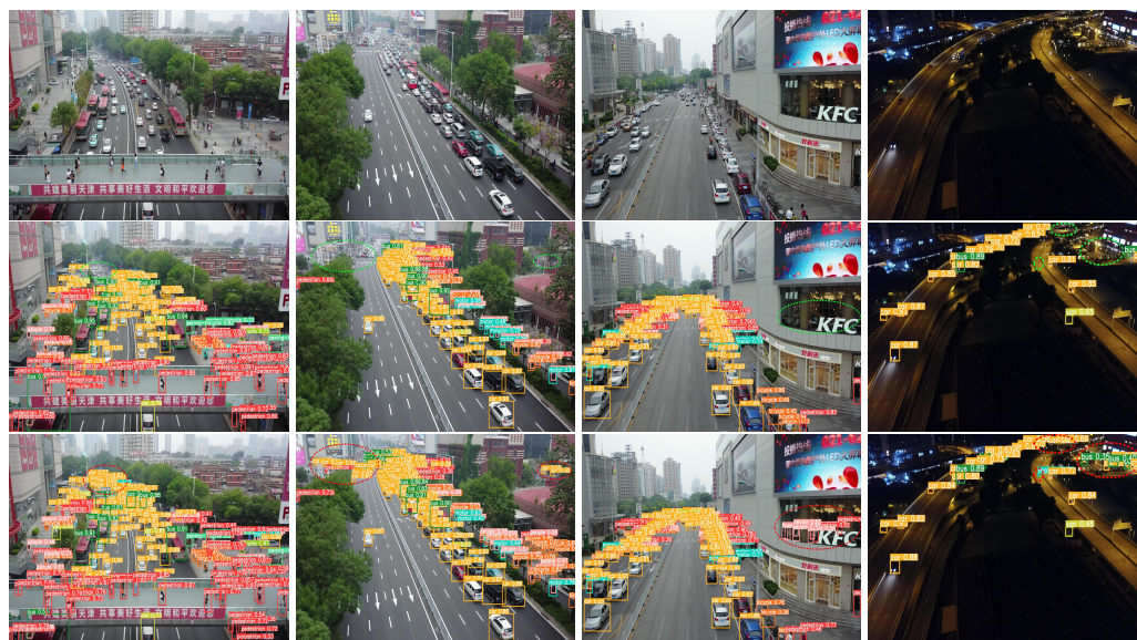
Figure 11. Some test results on the VisDrone2021-DET test. We selected some representative images for the display of the test results. The first row is the original image, the second row is the detection effect of YOLOv5x, and the third row is the detection result of Eagle-YOLO.
