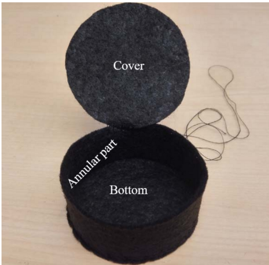
Figure 1: Full contact flexible mold for direct shear tests.
