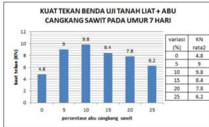
Gambar 3.23: Kuat Tekan Benda Uji Tanah Liat + Abu Cangkang Sawit 7 Hari
