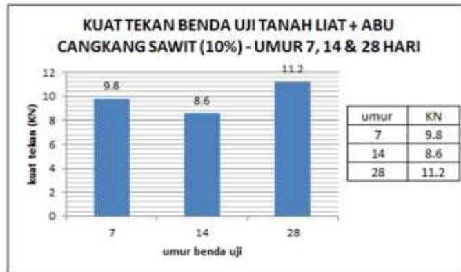
Gambar 3.17: Kuat Tekan Benda Uji Tanah Liat + Abu Cangkang Sawit (10%) – Umur 7, 14, 28 Hari
