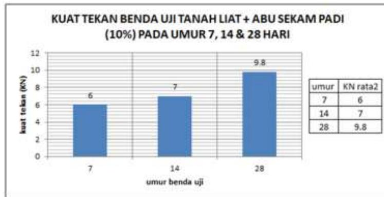
Gambar 3.6: Kuat Tekan Benda Uji Tanah Liat + ASP variasi 10%
