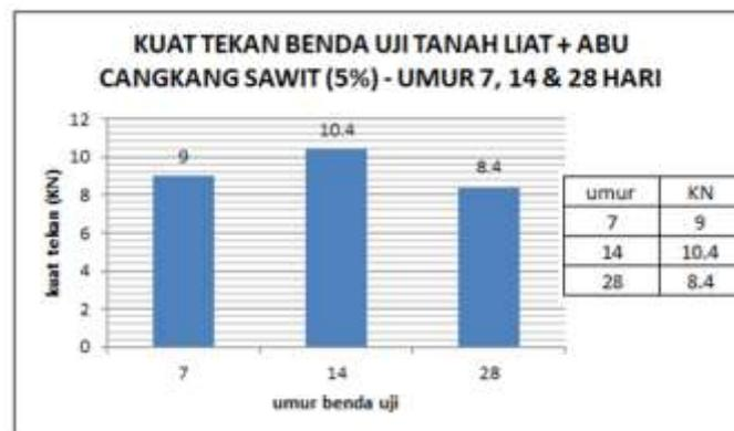
Gambar 3.16: Kuat Tekan Benda Uji Tanah Liat + Abu Cangkang Sawit (5%) – Umur 7, 14, 28 Hari
