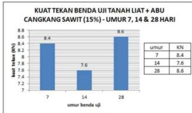
Gambar 3.19: Kuat Tekan Benda Uji Tanah Liat + Abu Cangkang Sawit (15%) – Umur 7, 14, 28 Hari
