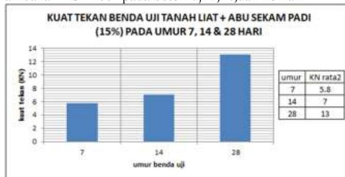
Gambar 3.7: Kuat Tekan Benda Uji Tanah Liat + ASP variasi 15%
