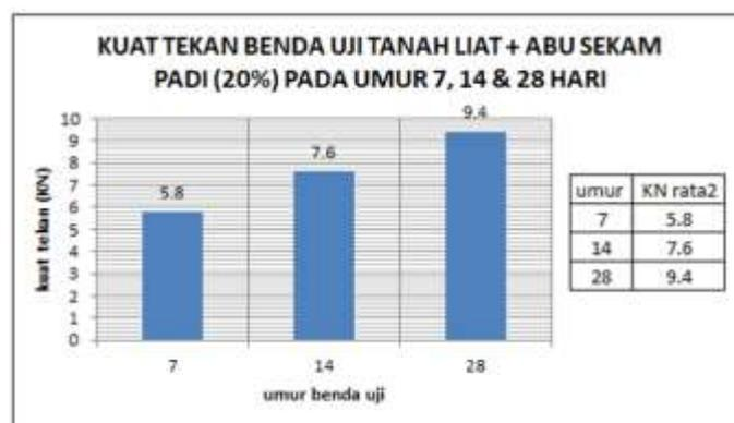
Gambar 3.8: Kuat Tekan Benda Uji Tanah Liat + ASP variasi 20%
