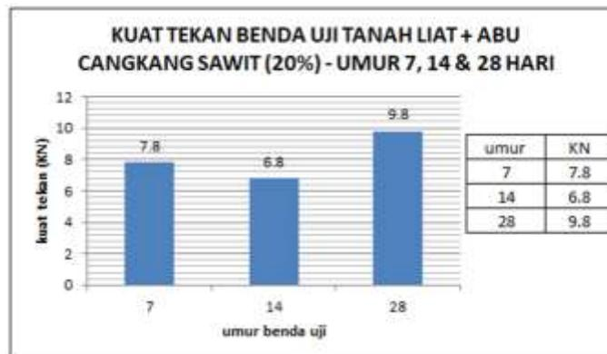
Gambar 3.20: Kuat Tekan Benda Uji Tanah Liat + Abu Cangkang Sawit (20%) – Umur 7, 14, 28 Hari
