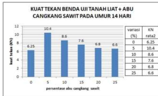
Gambar 3.24: Kuat Tekan Benda Uji Tanah Liat + Abu Cangkang Sawit 14 Hari
