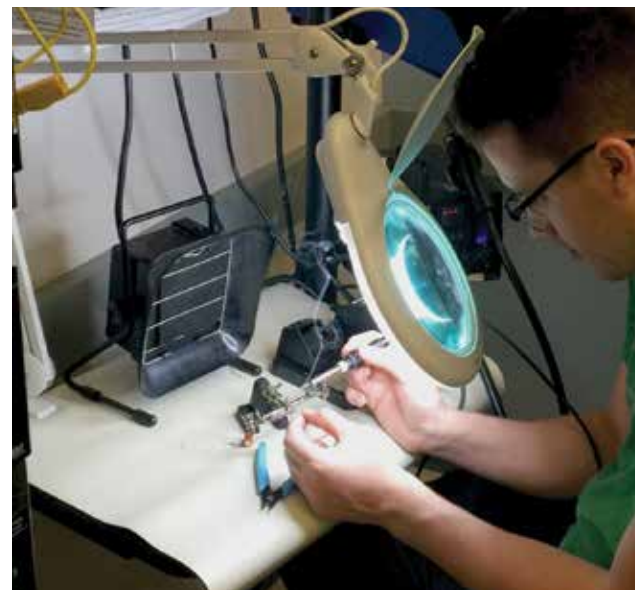
Peter Beery of ECE 17.1 soldering the power system monitoring device the team designed for Boeing.
