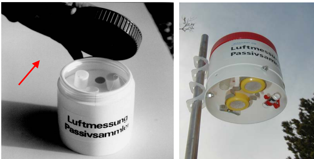
Figure 4.2: Passam protective shelter
