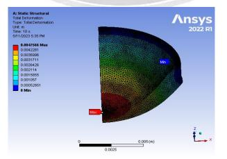
Fig. 12 Total Deformation for Neo-Hookean Model
