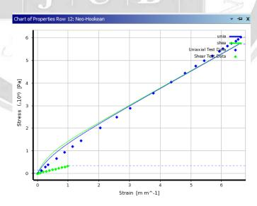
Fig. 5 Curve Fitting of Neo-Hookean based Material
