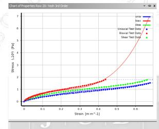
Fig. 6 Curve Fitting of Yeoh based Material
