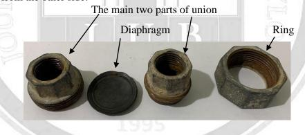
Fig. 23 Parts of Union Fitting with the Diaphragm
