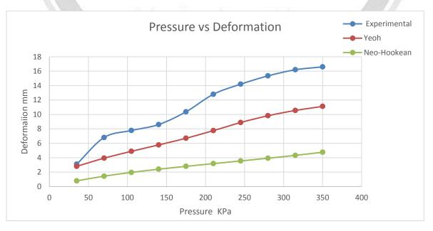
Fig. 27 Pressure vs Deformations
