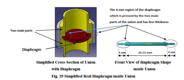
Due to pressing force on the edges of the diaphragm, the diaphragm might have initial 2. deformation prior to the deformation resulting in applied pressure by water.
