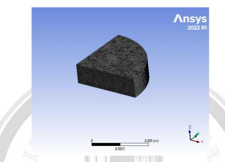
Fig. 7 Meshing of Neo-Hookean based Model
