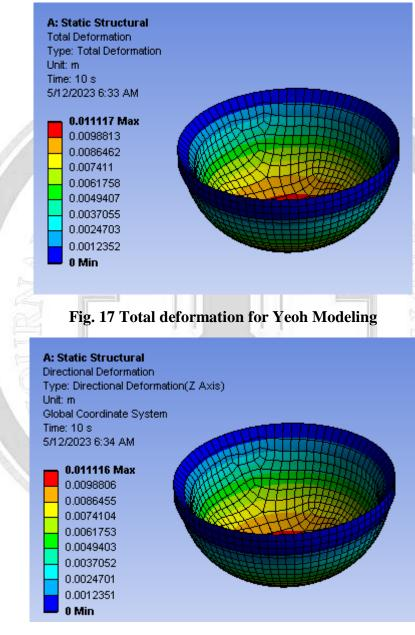
Fig. 18 directional deformation downward for Yeoh Modeling
