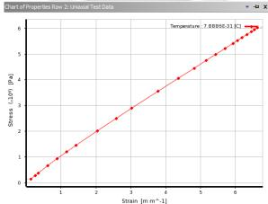
Fig. 4 Elastomer Sample (Neo-Hookean)
