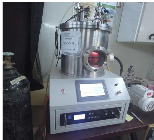
Figure(2):Composition of RF magnetron sputtering system.
