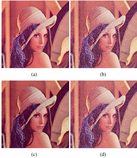
Fig. 2. (a) Lenna; (b) Noisy version of (a); (c) The erosion of image (b); (d) Linear mean filter of (b)
