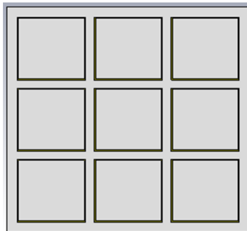
Figure 4. FSS periodical structure (3x3 array)
