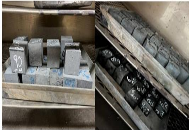
Figure 2. RPC cubes while curing
