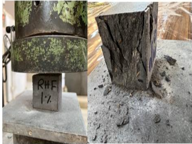
Figure 6. Testing of concrete sample
