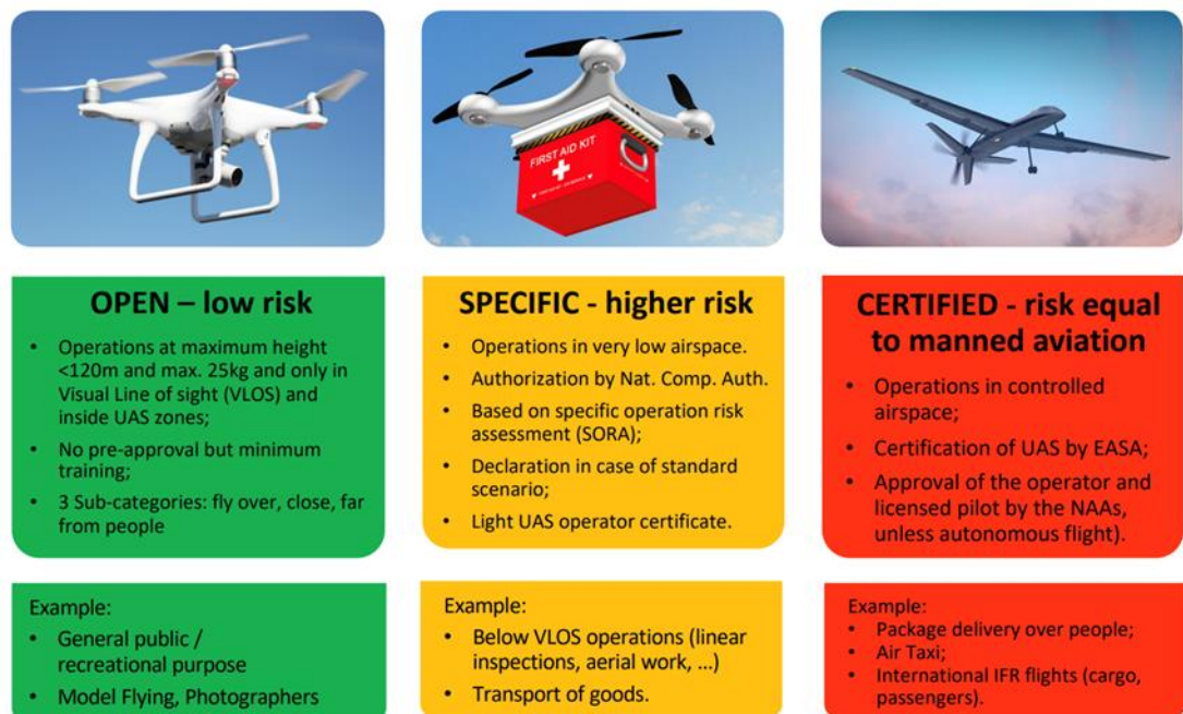
Figure 2. 2 Categories of Drone Operations Specified by European Rules on Drones (EASA, 2021)
