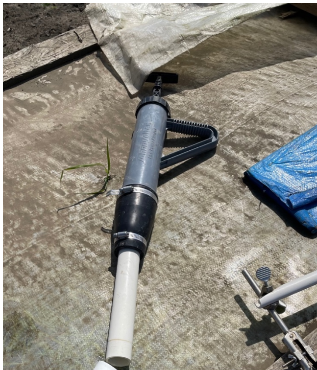
Figure 4. Picture of Johnny Jolter used to collect sediment samples from the bioreactor from 2020-2021.
