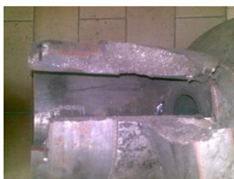
Gambar 5. Hub screw press in failure
