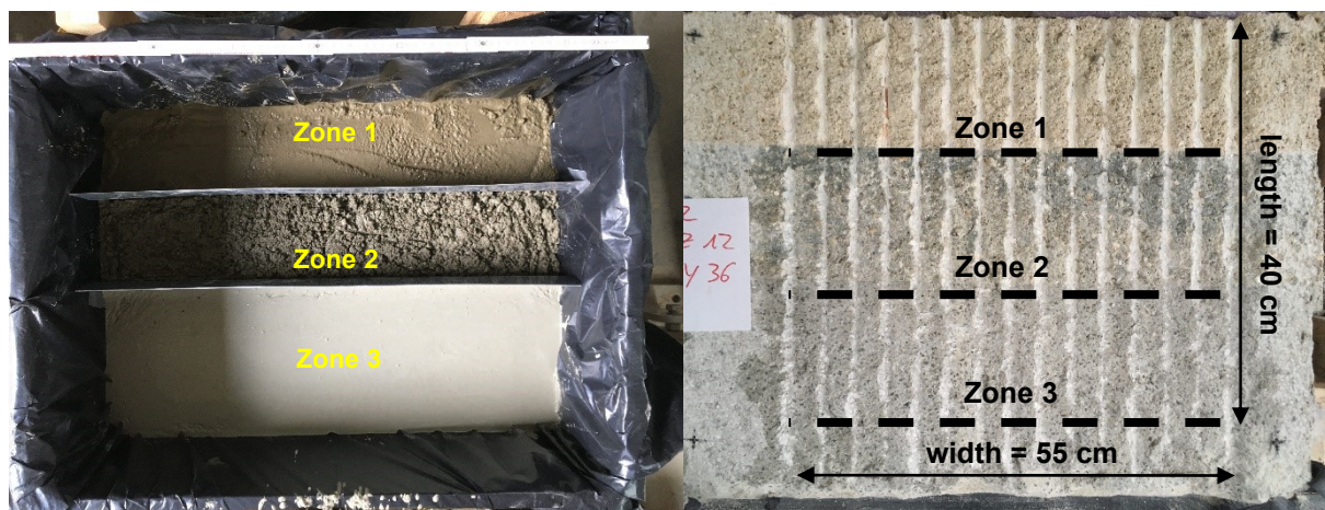
Figure 36: Zoning of test block during casting (left) and cutting (right)
