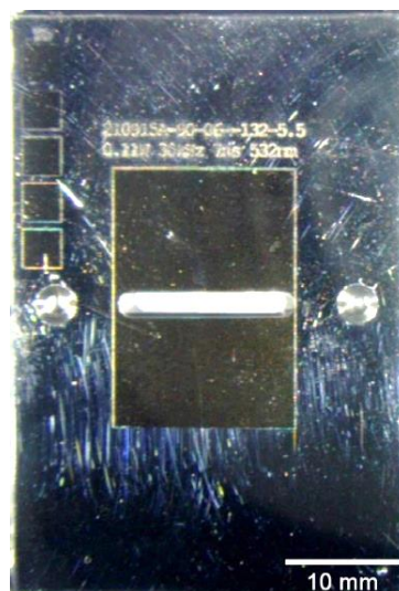
Figure 4.18: Optical image of an aperture plate after laser processing. The central darkened region above and below the central slot is a laser processed region with LIPPS features.
