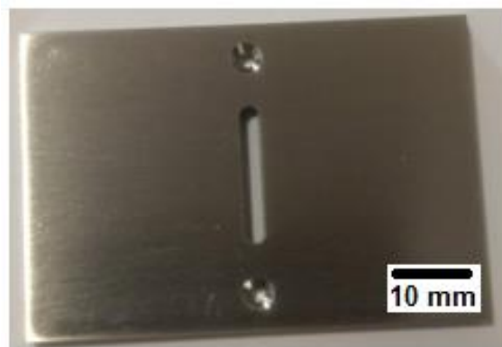
Figure 1.1: Optical image of the aperture plate electrode (design copyright Waters Corporation)
