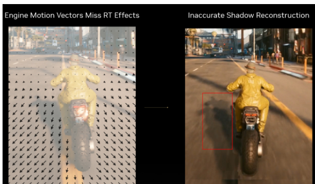
Figure 5. Frame generation with just motion vectors [6]
