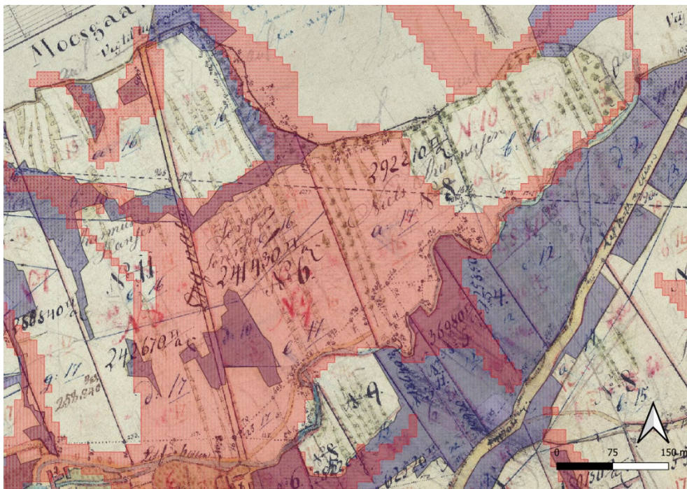
Fig. 10. Part of economic map (Danish: Udskiftningskort) dating 1783. A low-lying field is modelled as 'wet' (red raster), but is used as a tilled field. Recorded "meadow" on the cadastral map is shown (light blue). Notice there is evidence of furrows in the ridge-and-furrow system acting as surface drainage.
