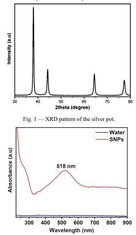
Fig. 2 — UV-Visible absorption spectrum of water and silver nanoparticles
