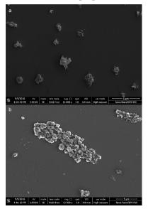
Fig. 3 — FESEM image of the silver nanoparticles with flowerlike morphology (a) as-prepared sample (b) after 24 h ageing
