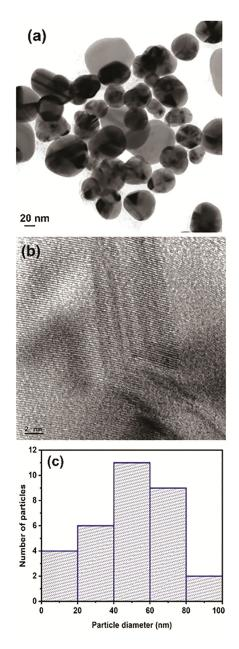
Fig. 8 — (a) The HR-TEM image (b) SAED pattern, and (c) particle size distribution of silver nanoparticles
