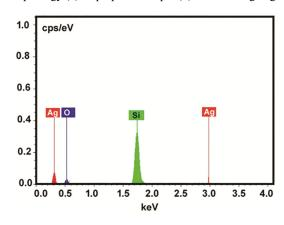
Fig. 4 — EDS of the silver nanoparticles
