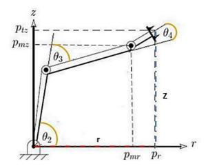
**Figure 3.** Geometric inverse of the Phantom in the ZR plane. Source: own elaboration.
