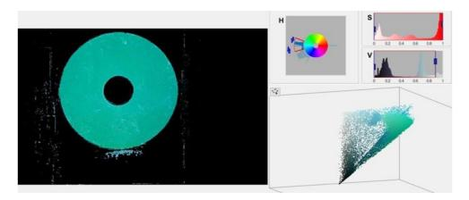
In the filtering by area, a threshold of 1000 pixels/in2 was used, resulting in the final segmentation shown in Figure 7.
