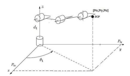
**Figure 2.** 3D geometric inverse of the Phantom. Source: own elaboration.
