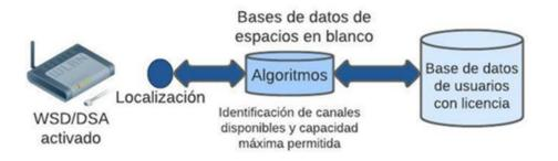
Figure 1: TVWS database access method. [16].
