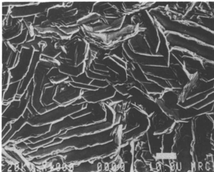
Fig.9 SEM photomicrograph for a deposit obtained with addition free electrolyte
