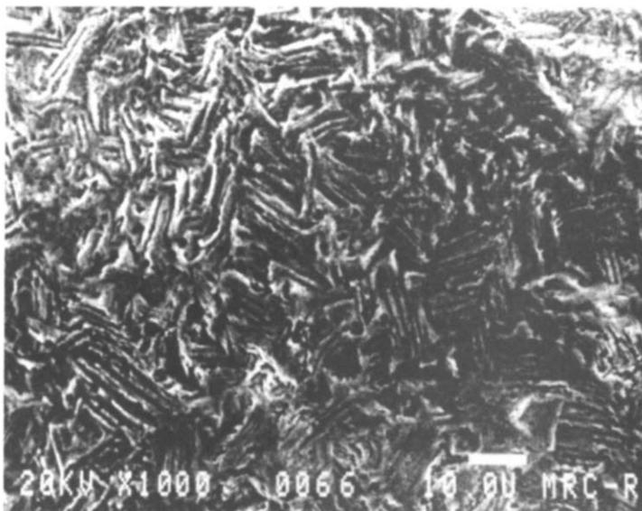
Fig.11 SEM photomicrograph for a deposit obtained from the electrolyte treated by four stage solvent extraction
