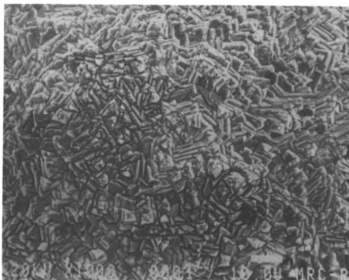
Fig.10 SEM photomicrograph for a deposit obtained with electrolyte containing 50 ppm D2EHPA
