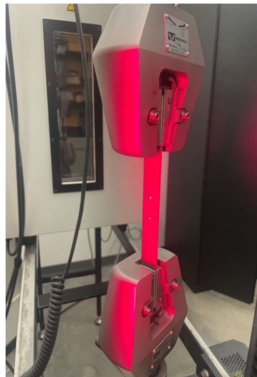
Figure 4. Flat Tensile Specimen Mounted on Instron
