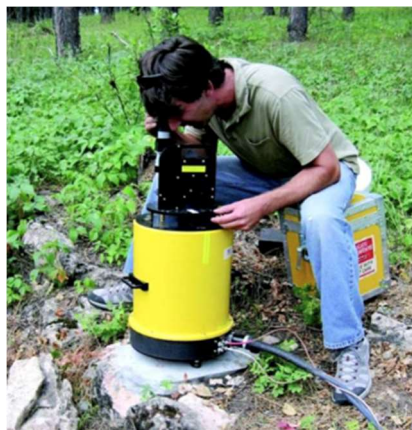
Figure 1: Image of a scientist using an absolute gravimeter at a base station in the Doty focus to the Northwest of Rapid City, SD. Microgravity measurements were collected for the purpose of determining changes in ground water storage in the karstic Madison aquifer in the Black Hills of South Dakota during 2009-12.4
