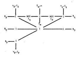
This model can be compared to the bond graph model of the synchronous machine by D. Sahn [7] which is shown below:
