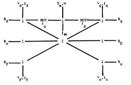
By using the ENPORT IV program, the power flow and causality are identified as:
