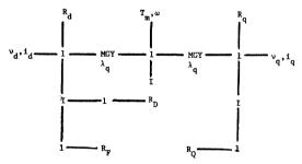
They are not alike. The model from [7] does not include the relationship to rotor speed and also does not include transformer action. Both of these characteristics are usually presented in the conventional model of the induction machine, otherwise they would be equivalent.
