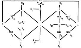
By using the ENPORT IV program, the power flow and causalities are identified as:
