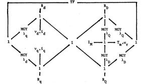
The bond graph model of the induction machine given by D. Sahn [7] is
