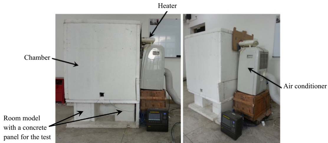
b) Self-designed environmental chamber with heater and air conditioner
