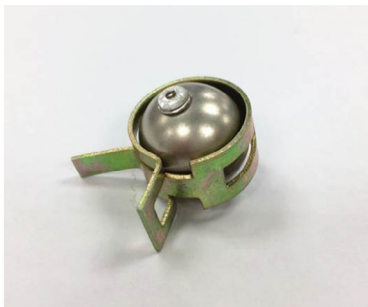
c) HSB attached with metal clamp (PCM-HSB-c)
