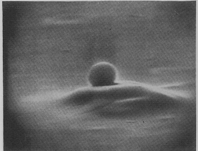
Figure 8. SEM micrograph of 0.5- \mu\text{m} diameter latex particle and a Liesegang circle scanned at a zenith angle of 85°.
