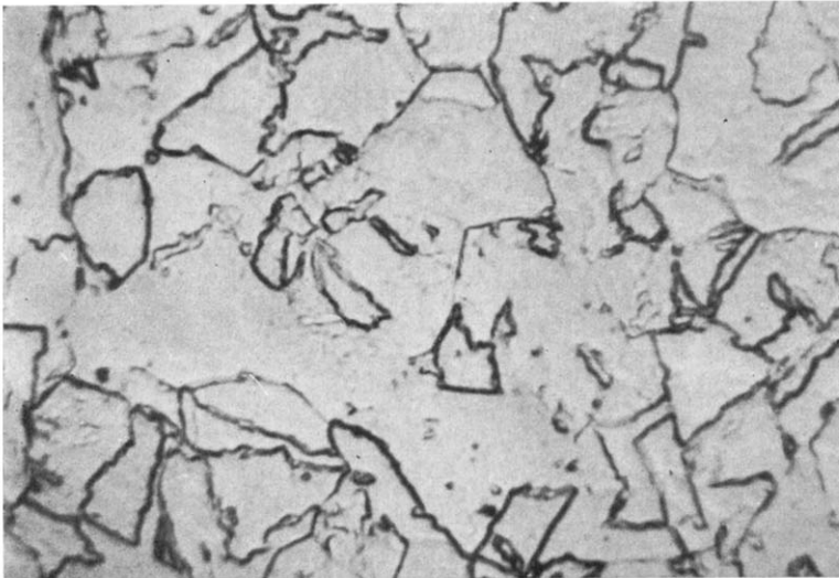
FIG. B.12. Maraging steel. \times 250
