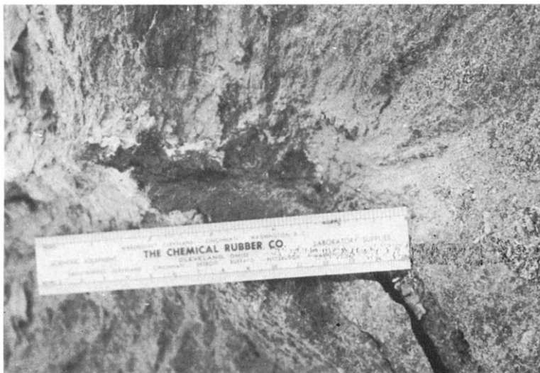
FIG. 16. Longitudinal section of the shaped charge hole.
