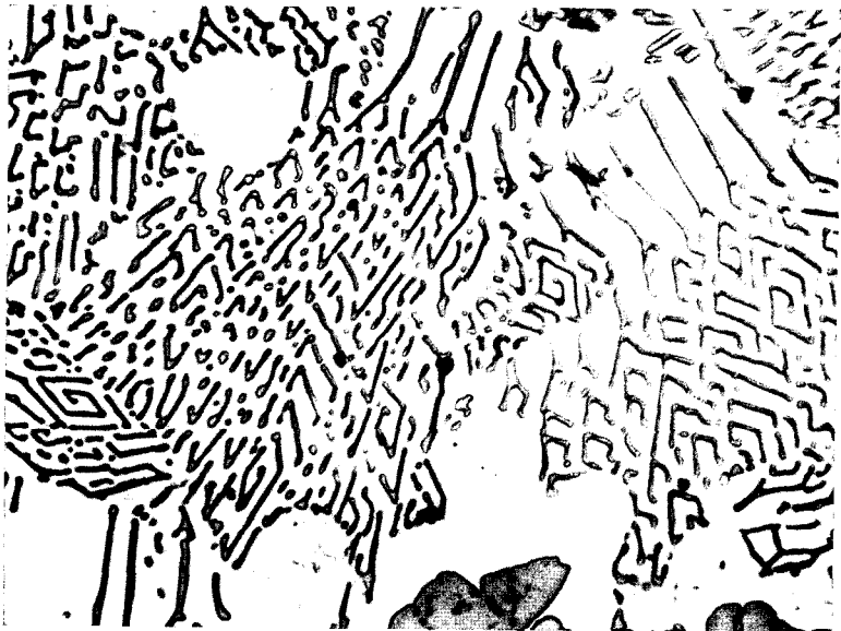
FIG. 13. Photomicrograph showing eutectic spiral formation in a aluminum-25 weight percent uranium alloy. 1000 \times .
