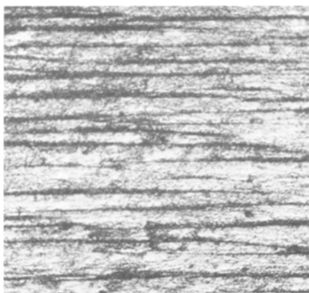
Fig. 2. Crystallite of zone-refined Fe. Etchant: conc. HCl, 12 hr. 150X.
