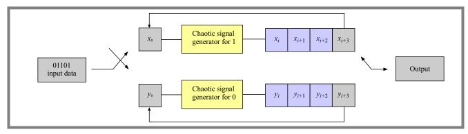
Fig. 3. CSK encoder proposed for error correction.
