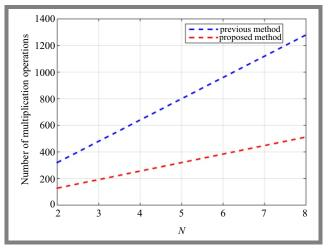
Fig. 13. Proposed and existing error correction method versus N parameter.
