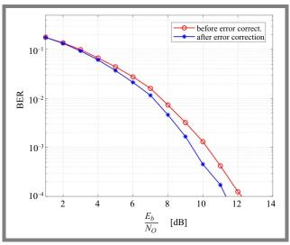
Fig. 11. BER after and before error correction,  $N_d = 4$ .
