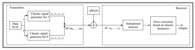
Fig. 1. CSK system with the proposed error correction coding scheme.
