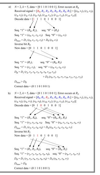
**Fig. 9.** Error correction algorithm used in the proposed approach: a) error occurs in the first bit, b) error occurs in the third bit.
