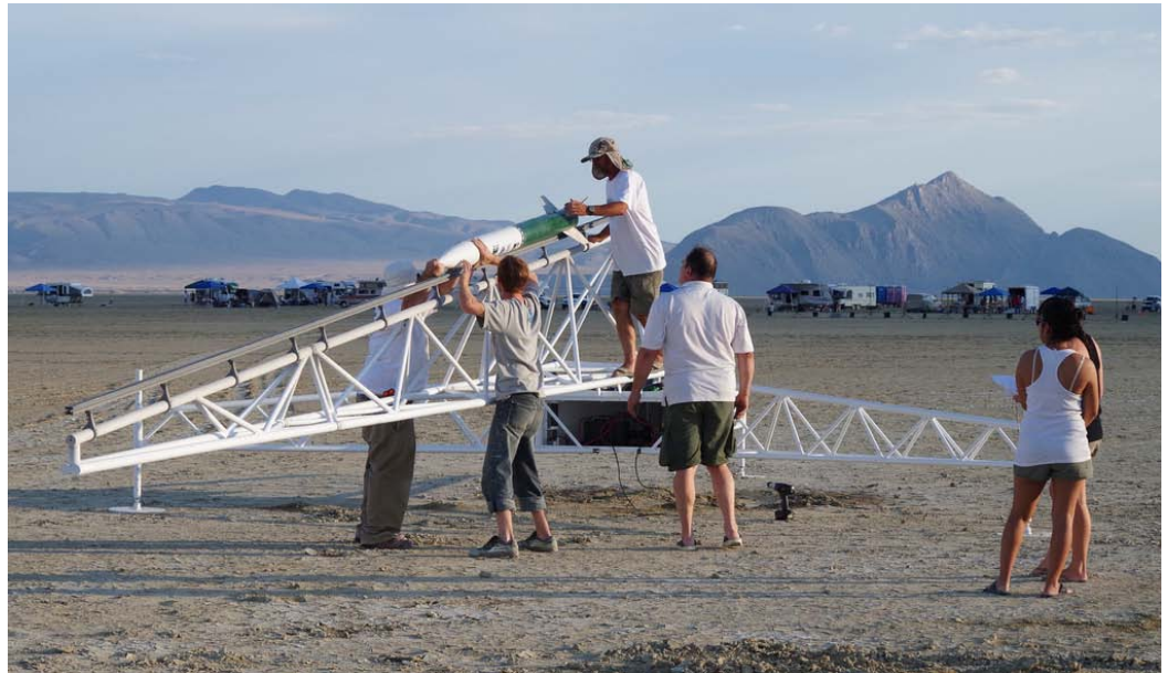
ARLISS team members readying a rocket for launch by loading it onto the launch rail. The rail will be lifted vertically once the rocket is ready.
