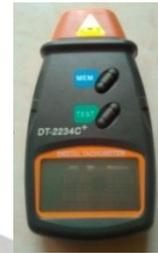
Gambar 7. Tachometer digital
