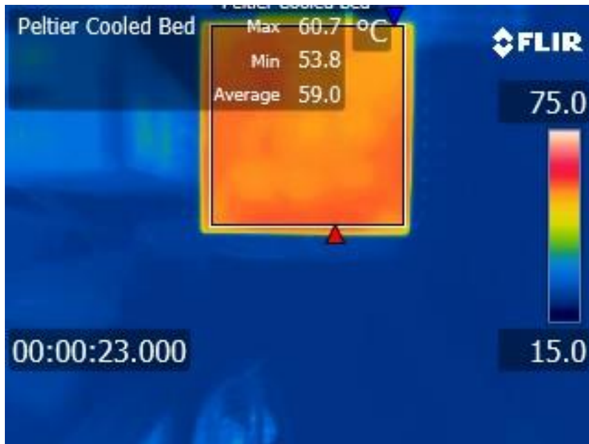
Figure 16: Peltier Cooling FLIR Camera Snapshot
