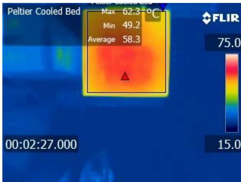
Figure 17: Peltier Cooling Heat Bleed FLIR Camera Snapshot
