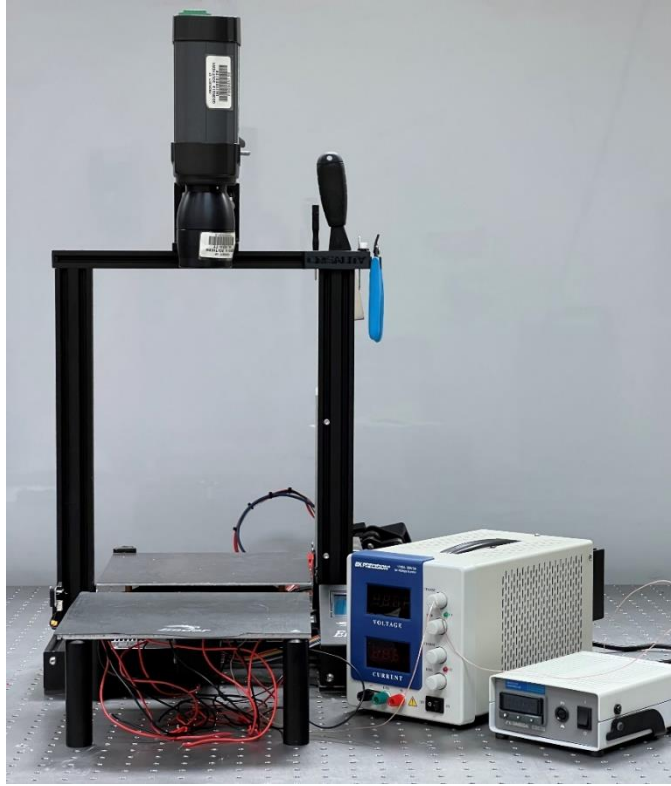
Figure 4: Peltier Heating and Cooling Experimental Setup
