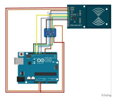
Figure 11. ATRAPPMAN Wiring Diagram
