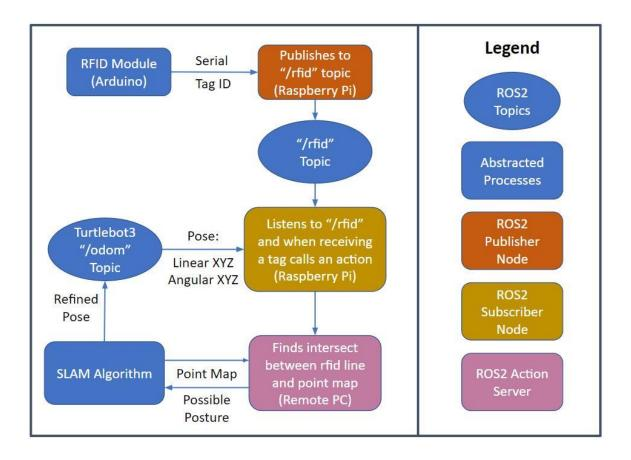
Figure 12. Control Architecture Flow Chart
