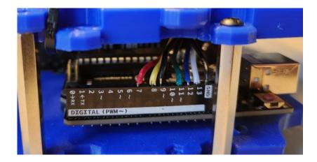
Figure 15. Arduino Pin Locations
