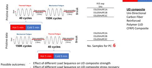
Figure 2. Effect of Thermal/Mechanical Fatigue Load Sequence on UD Composites
