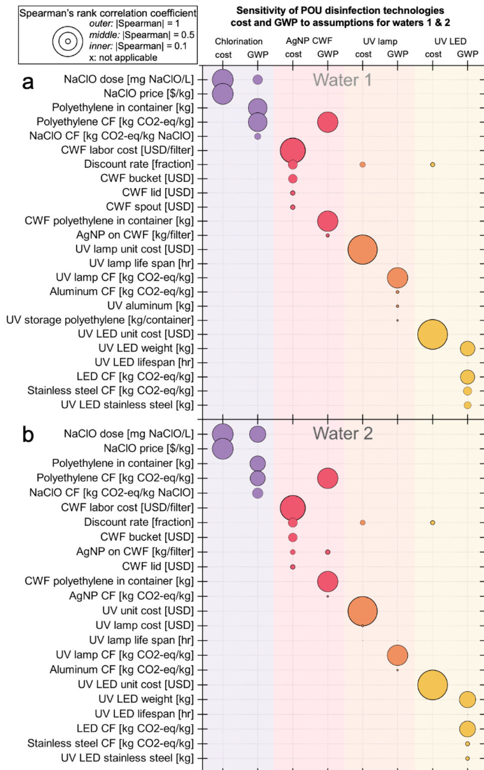
Figure 14. Spearman's rank correlation for net cost and GWP for all POU technologies with water type 1 (a) and water type 2 (b). The key drivers are on the ordinate corresponding with each technology's cost and GWP on the abscissa.
