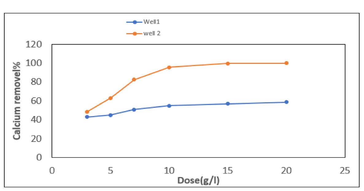
Fig.6. Effect of soda ash dosage on calcium removal in the
