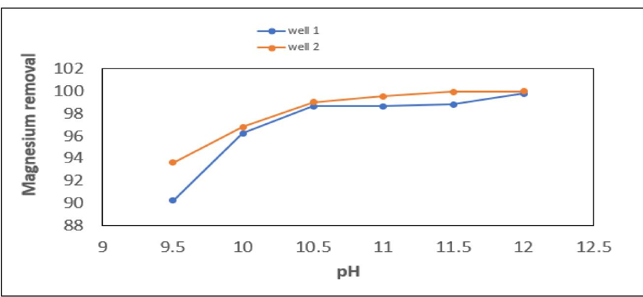
Fig.5. Effect of pH on magnesium removal in produced water.
