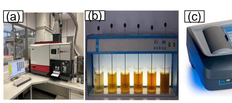
Fig4: (a) ICP/OES, (b) Jar Test, (c) Spectrophotometer
