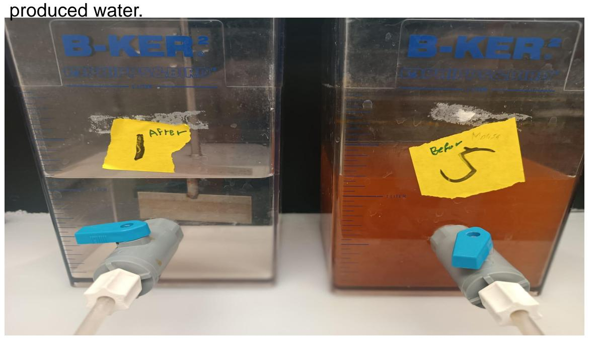
Fig.7. Effect of pH on magnesium removal in produced water.
