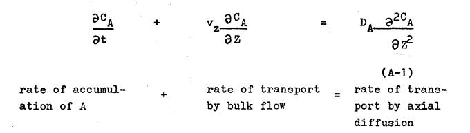
Since both solid and liquid phases are present, let  $\ell$  be the fraction of volume occupied by the liquid, and let  $\partial C_{Af}/\partial t$  and  $\partial C_{As}/\partial t$  be the rate of accumulation of A in the liquid and solid phases respectively. Eq. (A-1) then becomes,
