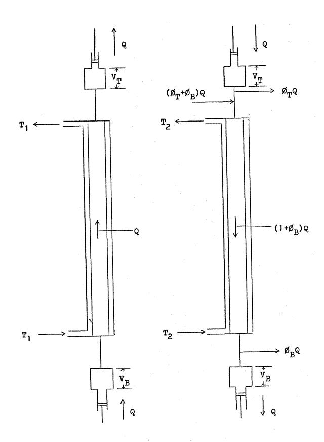
Figure B-3 — The Semicontinuous Parametric Pump
