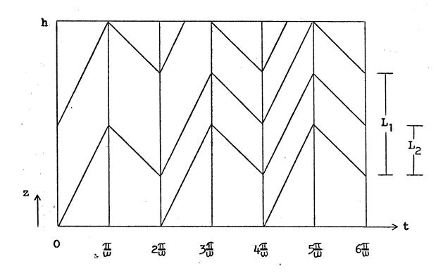
Figure B-1 — Concentration Front Characteristics for Region One
