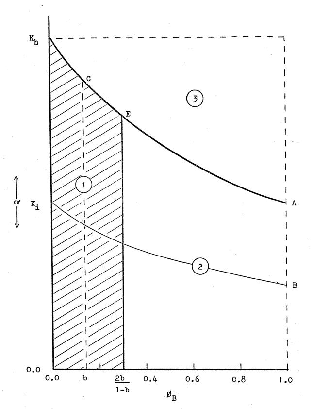
Figure 8 — The Three Regions of Operation Viewed on the  $Q-\emptyset_B$ Plane for the Semicontinuous Mode
