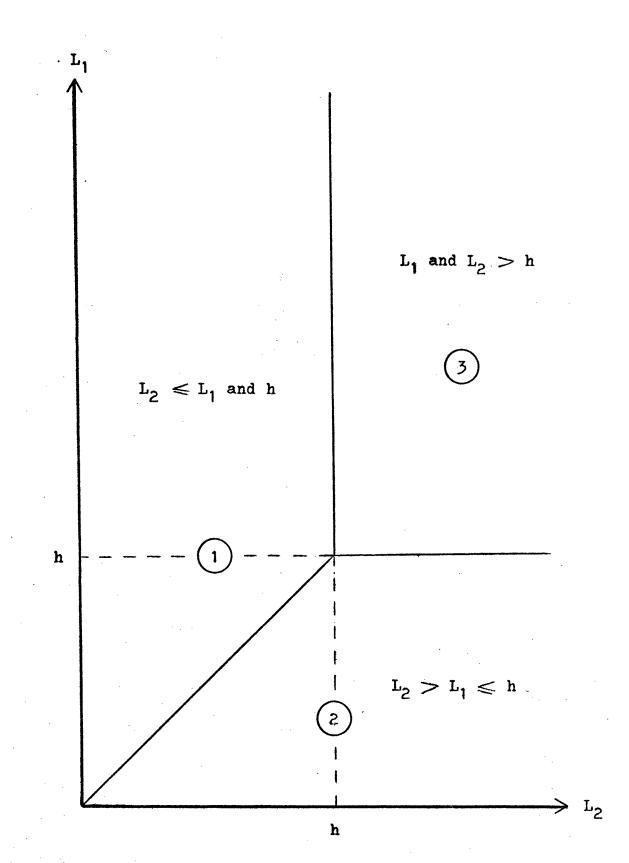
Figure B-4 - The Three Regions of Parametric Pump Operation
