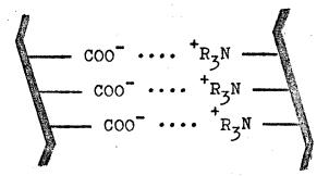
where the solid curved lines represent the organic polymer lattice. Inorganic ions are adsorbed with a mechanism differing from that of conventional ion exchange shown by the following:
