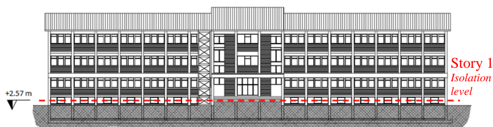
Figure 8. Position of the isolation level (red dashed line) with location of the single-concave FP devices. 265 266
