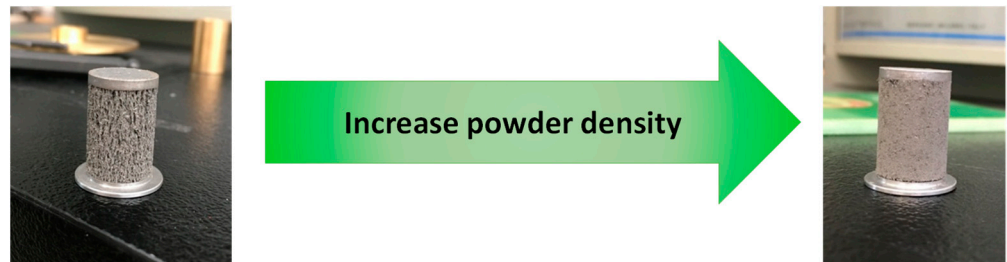
Figure 11. The density variation for the same volume cylinder of recycled NdFeB powder.
